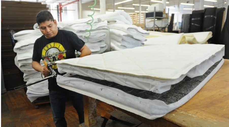
Marelo Mejia uses a pneumatic staple gun in building a box spring to a customer's exact specifications.
