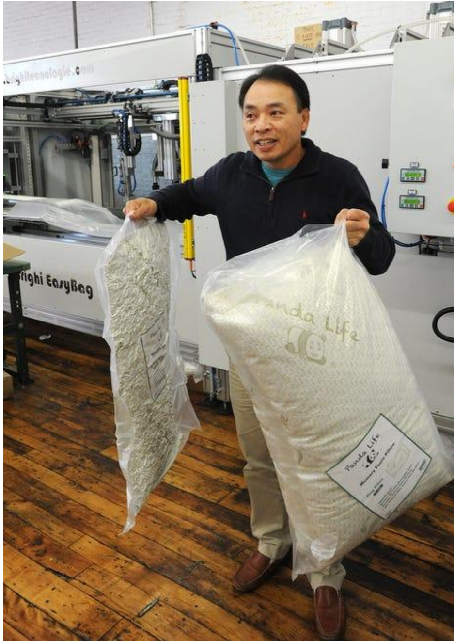
U.S. Bedding President and CEO David Nguyen shows how two memory foam pillows can shrink in size after a machine squeezes the air out of them and seals them for shipping.
