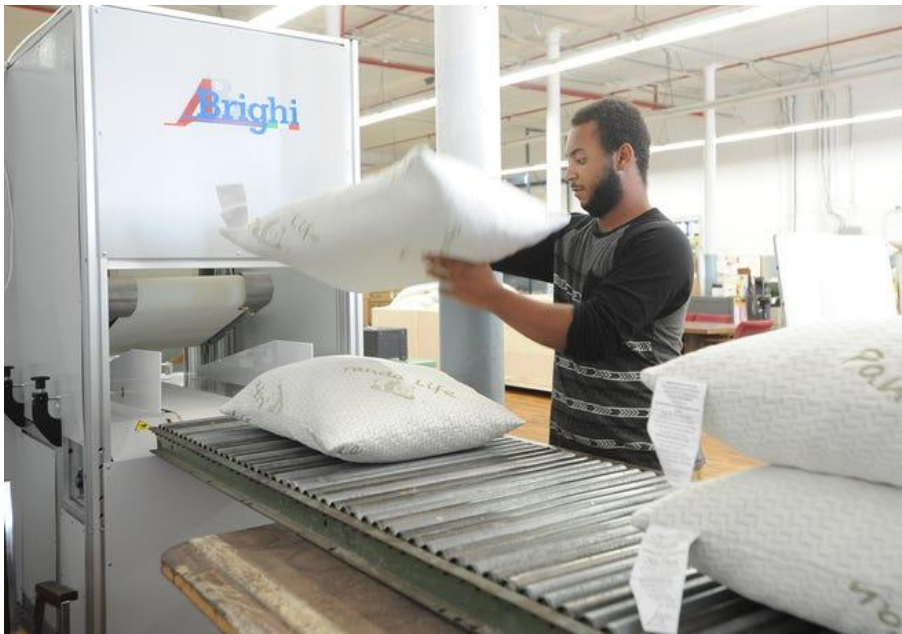
At U.S. Bedding, Eddie Lima runs a machine that crushes the air out of memory foam pillows for shipping.
